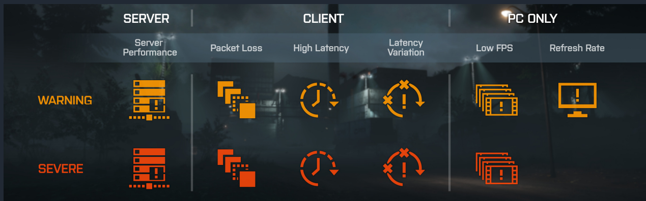
Server performance, Packet loss, High latency, Latency Variation, Framerate and Screen update rate warning icons
